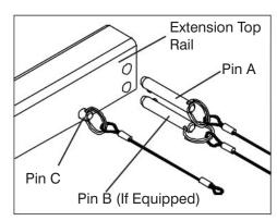
Figure 3-13b. Extension Top Rail Pins
