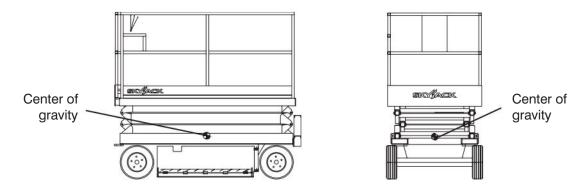
Figure 3-15. Center of Gravity
