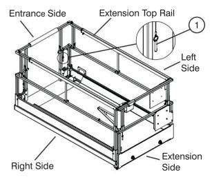
Figure 3-13a. Folding Guardrail System
