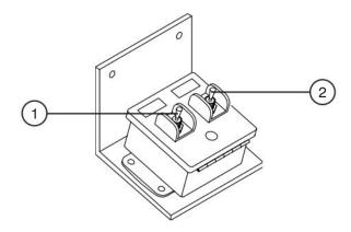
Figure 3-8. Powered Extension Control Console
