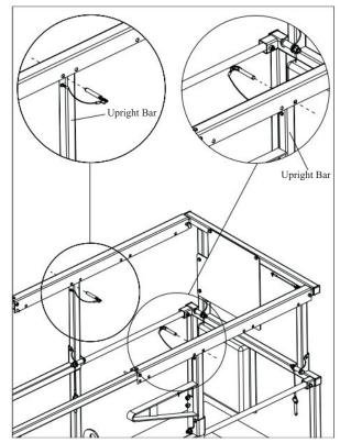
Figure 3-12. Variable Position Manual Extension
