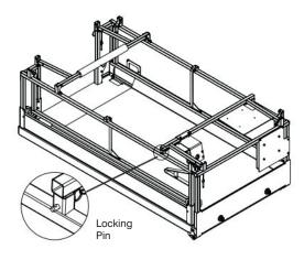
Figure 3-13c. All Guardrails Folded Down
